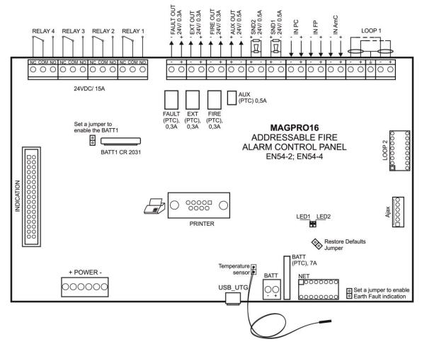
Figure 7 – Main PCB of the MAGPRO16 fire alarm panel
