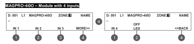
The input numbers correspond to the functional number buttons. The programming is same for all of the inputs. For the settings of the 'IN 1/2/3/4' refer to the submenu of MAGPRO-Mini. (2) ON/ OFF LED – Press to switch on/ off the device LED.
