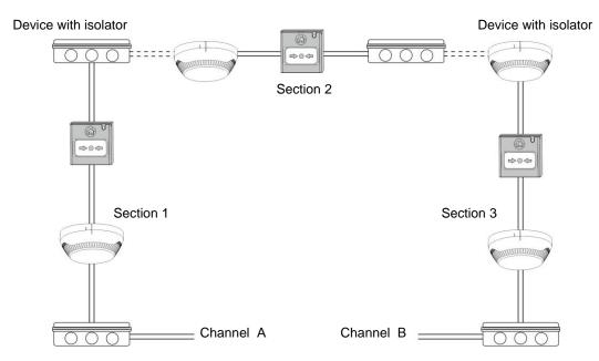
Figure 15 – Example for connecting of detectors and call points to a loop expander (the built-in in the main control panel or MAGPRO16-L250 Loop)
