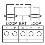
Figure 9 - Connection to the loop controller
