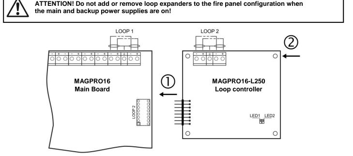
① - Connect the connectors: LOOP 2 of the main control panel and LOOP of the second loop controller.
