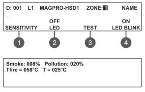
Use the functional buttons to set the following parameters: (1) **SENSITIVITY** – Press to set the sensitivity of the smoke chamber for DAY and NIGHT alarm mode (see the description of MAGPRO-SD1). The set sensitivity levels are confirmed wit ENTER button.
