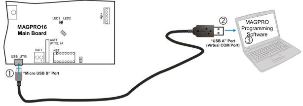
Figure 20. Programming via MAGPRO programming software
