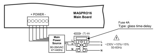
Figure 16. Connecting the main power supply cable to the 230V terminal
