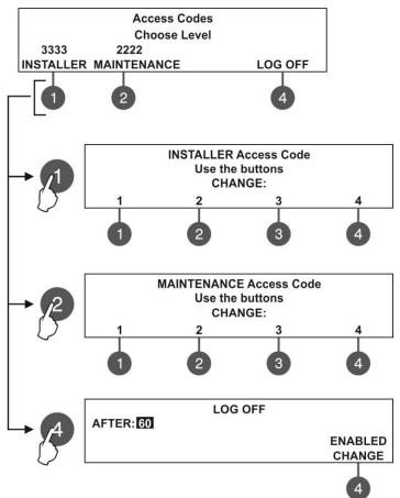
The settings are analogical for both levels. Use the functional buttons to set access code for: (1) - Press to change INSTALLER CODE
