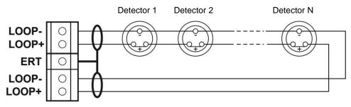
Figure 13 – Connecting of detectors to a loop controller
